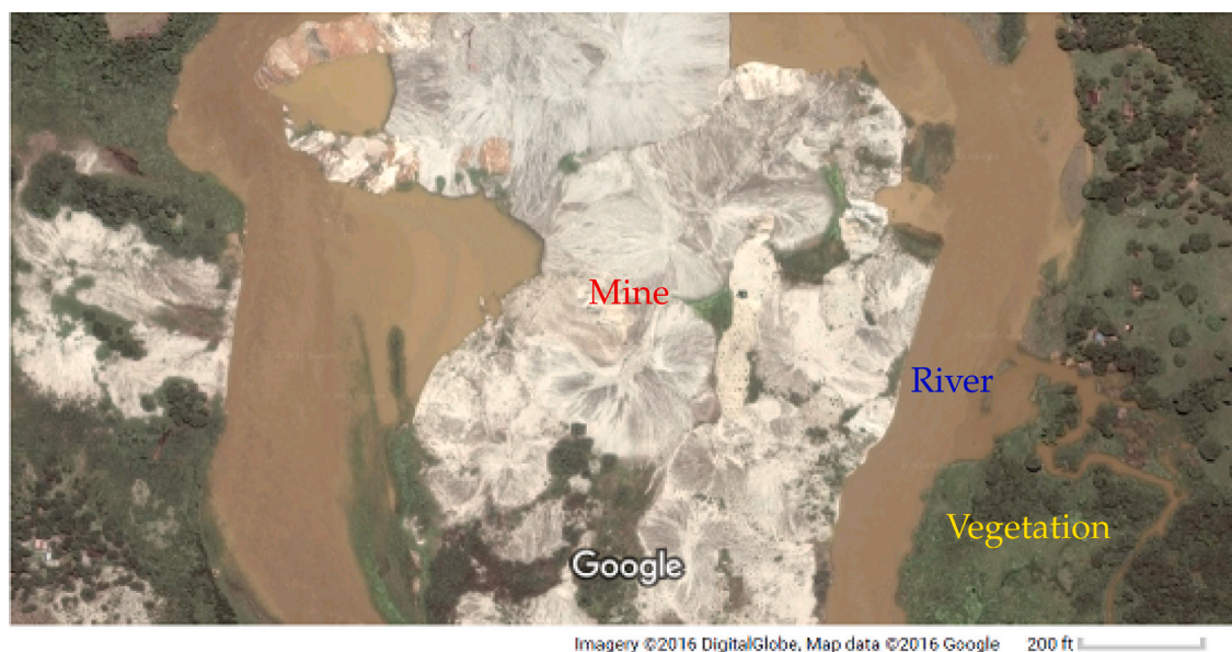
Fig. 2. Image of the footprint of a mine. Notes: Example of a mine we aim to detect with the machine learning algorithm. The white portion of the image is the mine footprint, in contrast to the river (brown) and vegetation (green). (For interpretation of the references to color in this figure legend, the reader is referred to the web version of this article.)
